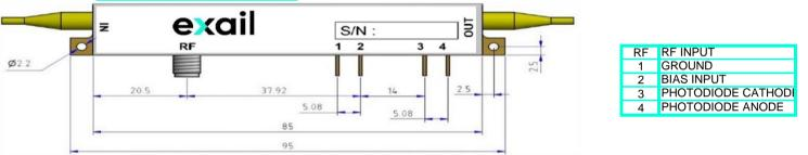
Thickness : 9.6mm Material : KOVAR Package dimensions in mm
