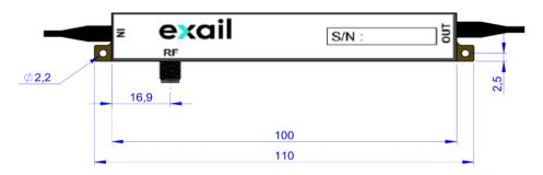
Thickness: 9.6mm Material: INOX 304L Package dimensions in mm
