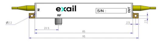
Thickness: 9.6mm Material: KOVAR Package dimensions in mm
