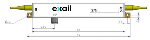
Thickness: 9.6mm Material: KOVAR Package dimensions in mm
