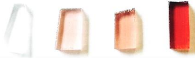
Figure 2 : Visualization of Radiation Induced Attenuation (RIA) on glass irradiated by 6 MeV electrons at room temperature. From left to right: pristine glass, 600 Gy(SiO 2 ), 1 kGy(SiO 2 ), and 5 kGy(SiO 2 ), from [2].
